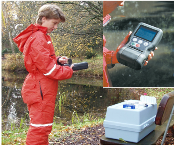
Figure 1.4 HACH-LANGE ECLOX Handheld Luminometer.
